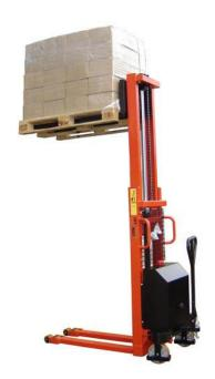
This stacker has electric lift and lowering and is capable of lifting up to 500kg to a height of either 1600mm or 3500mm.
