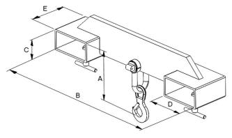
Adjustable Fork Mounted Hooks are the most cost effective way of safely hanging a load under the forks of your lift truck. Simply clamps on the forks anywhere along there length.
