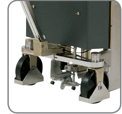
EHS 1000 RF-SEMI has assisted wheel steering. Easy and hygienic operations.
