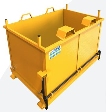
A simple but effective means of collecting, moving and safely dumping factory waste. These containers dump the waste through the base, which opens by means of a pull-cord. The base automatically re-locks when lowered onto a hard surface. Can also be supplied with castors and lids if required.
